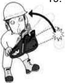
19. Guard against kickback. Kickback is the upward motion of the guide bar which occurs when the saw chain at the nose of the guide bar contacts an object. Kickback can lead to dangerous loss of control of the chain saw.
